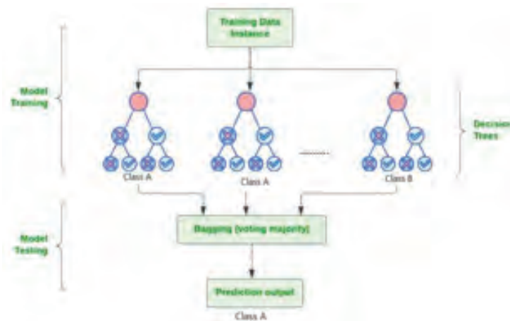
Figure 4: Shows the training methodology of Random Forest algorithm. It majorly works with decision trees.
